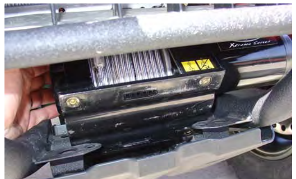
"Figure 4" Rotate Winch Utilizing The Space Between The Mounting Tabs
