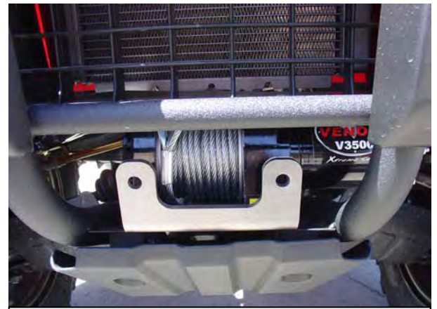
“Figure 5” Put Winch Mount Into Location
