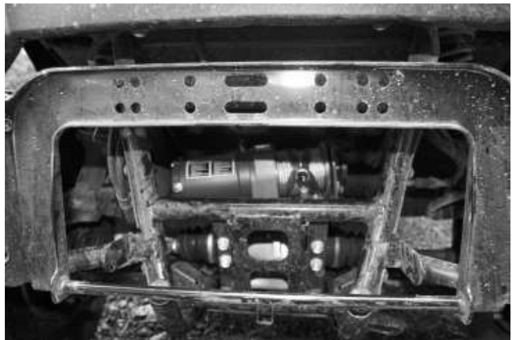
Figure 2 Place Winch Inside The UTV Frame
