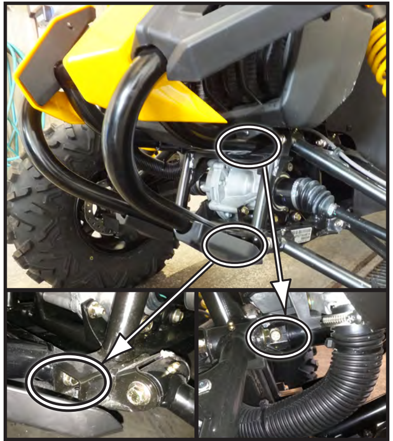
“Figure 2” Bumper Removal
