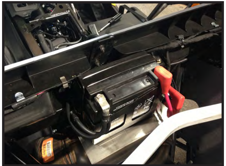
“Figure 8” Battery Location (Battery is located under panel in the bed.)
