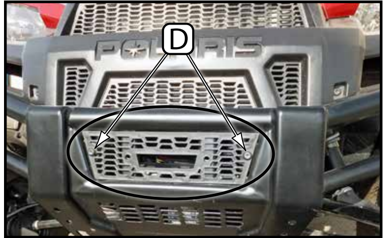
“Figure 4” Bumper Grill Removal
