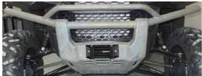
"Figure 10" Fairlead install (Wide Fairlead)
