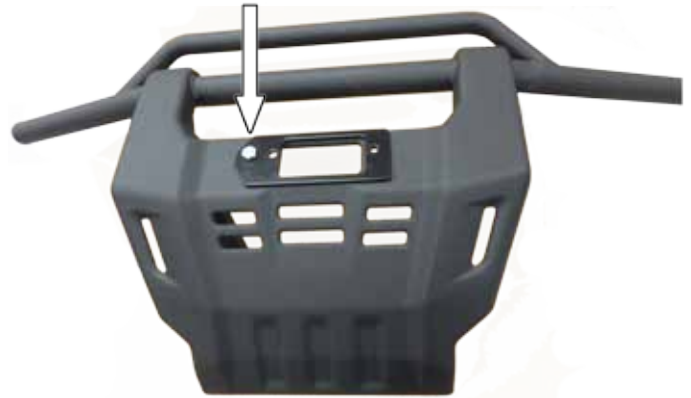
"Figure 8" Fairlead Mount Plate install (Standard Fairlead)
