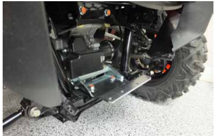
“Figure 5” Mount support bracket attached with supplied hardware
