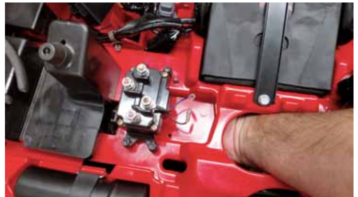
“Figure 12” Contactor installation
