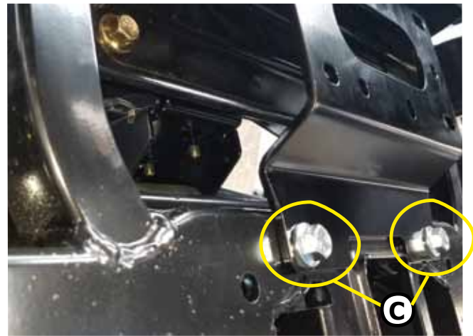
"Figure 3" Lower Winch Mount Bolts
