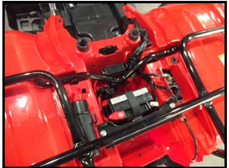
“Figure 8” Battery Location (Battery is located under the plastic panel behind seat.)
