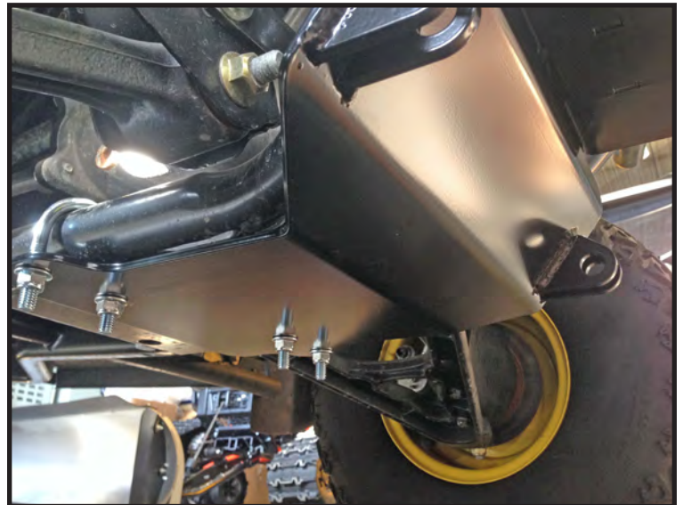
“Figure 3” U-Bolt Install
