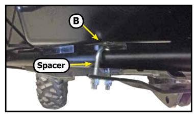
"Figure 5" Spacer Install
