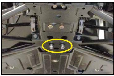
"Figure 2" Bolt Plate Install Location
