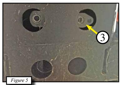
5. Hold the rear of the frame bracket (1) to the frame and loosely attach using two bolts (4), lock washers, and washers into the bolt plate (3). Shown in Figures 5 & 6.
