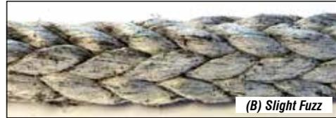
Once approximately 25% of the outer fibers show wear (see Figure C), the cable must be replaced.
