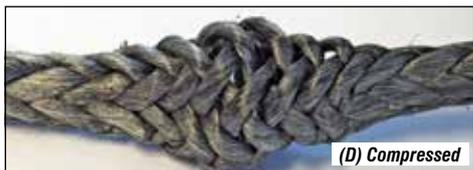
Look for powdered fiber or abrasion (signs of internal wear). Consider the amount of wear on the internal fibers when determining the percent of wear for replacement.
