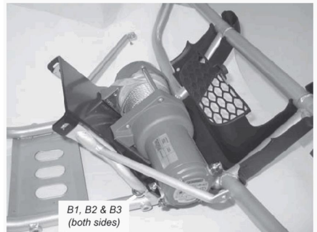
Figure 7 Place Mounting Plate, Fairlead, and Winch onto front Bumper
