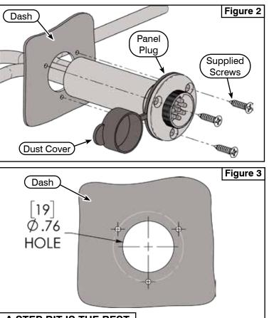
A STEP BIT IS THE BEST OPTION FOR MAKING THIS HOLE. AFTER PRINTING, LINE BELOW SHOULD MEASURE 1" - 1"-
